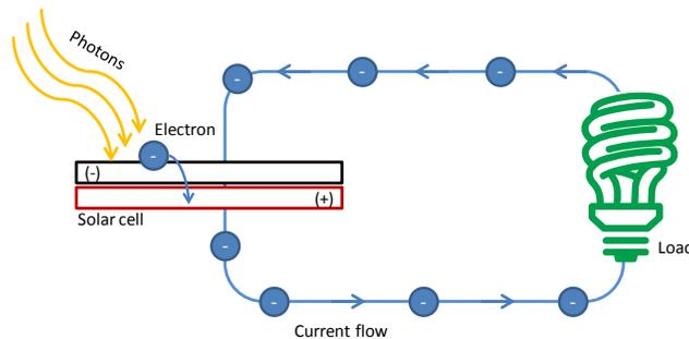
**Figure 2. Generation of electricity from a PV cell**
