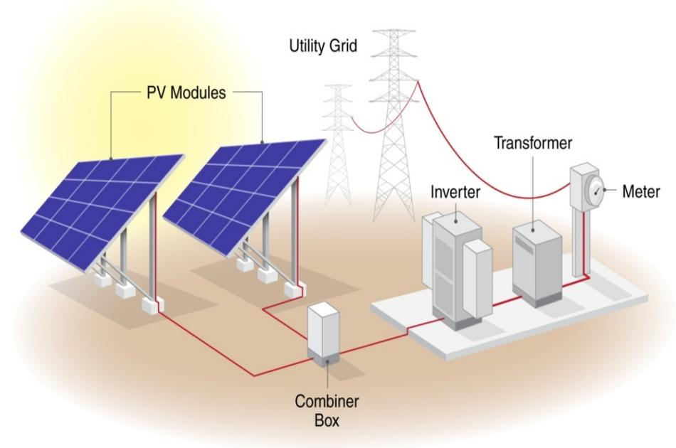
**Figure 3. Ground-mounted array diagram**
